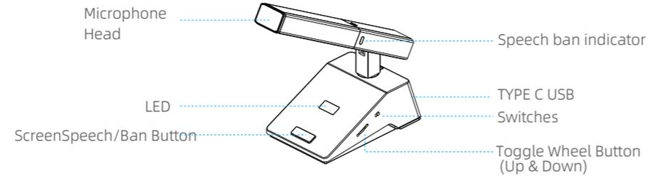
Product built-in rechargeable lithium battery, provide charging interface, can continue to speak for 10 hours or continuous 24 hours of standby work, and the use of unique encryption technology to ensure that the meeting information security; equipped with LCD display, real-time display call volume, call status, circuit status, with independent gain adjustment, speech timing function, support three role definition: the chairman \VIP \ listed.
